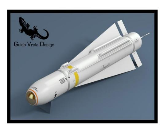
One of the missiles used commonly is the AGM-65 Maverick. The mayerick ia a air-to-surface missile it is a commonly used munition for the A-10, targeted via electro-optical (TV-guided). Other weapons include <u>cluster bombs</u> and <u>Hydra</u> rocket pods. The A-10 is equipped to carry GPS and laser-quided bombs, such as the GBU-39 Small Diameter Bomb
